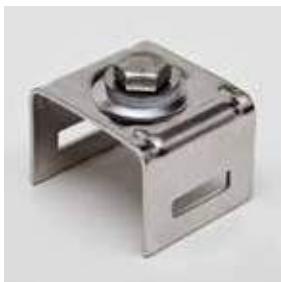
SINGLE BOLT STRAP BRACKET - LARGE DIA. POLES Manufactured using high strength stainless steel and metal forming technology that adds reinforced ribbing for additional strength. D5-SS-SSB-RND4L
